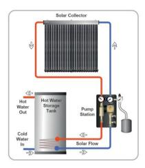
The dedicated solar hot water heating system can be a single tank (as illustrated above) or a dedicated solar tank can provide pre-heated water to a main hot water tank.
